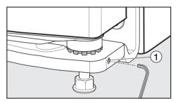
Unscrew threaded pin ④ by one half of a turn using the allen key supplied.
